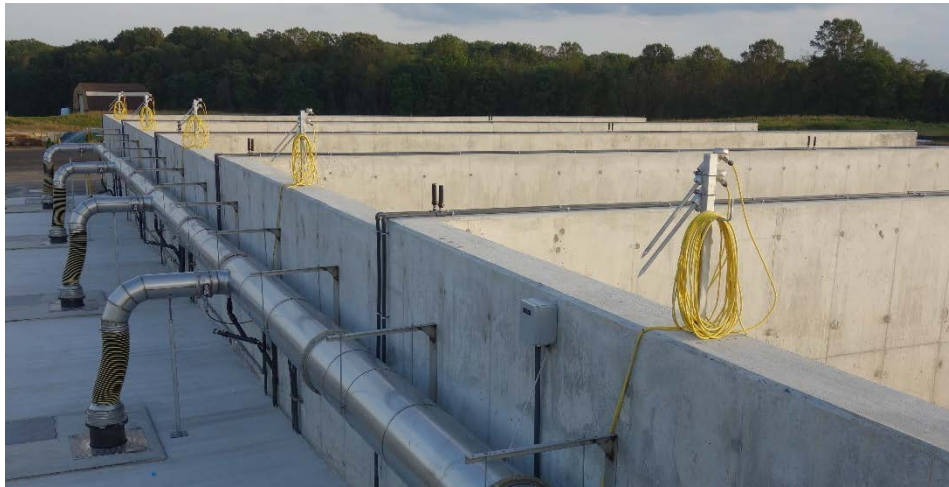
Figure 4: Temperature probes in storage racks on top of push wall
