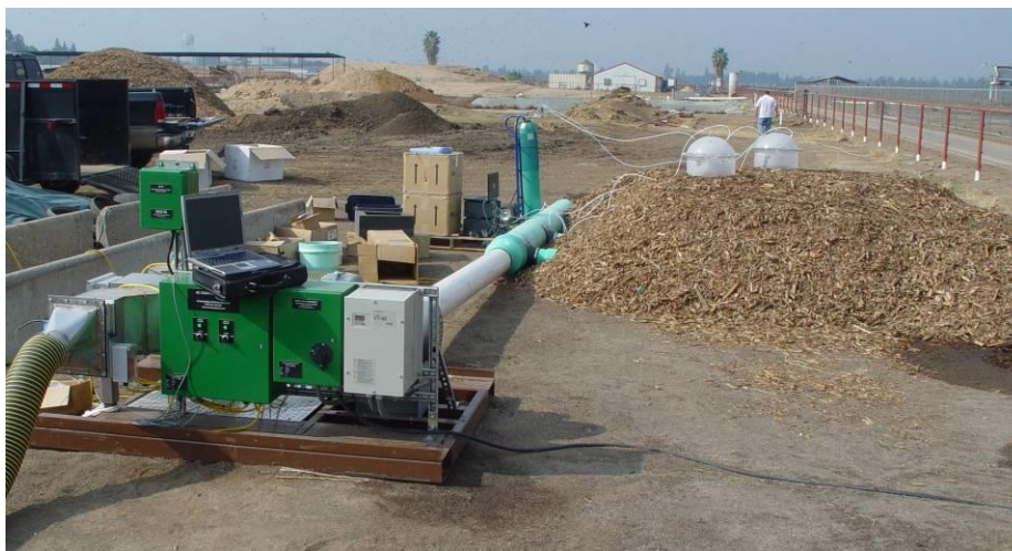
Photo 2- Negative CASP Pilot Biofilter Emissions Testing
