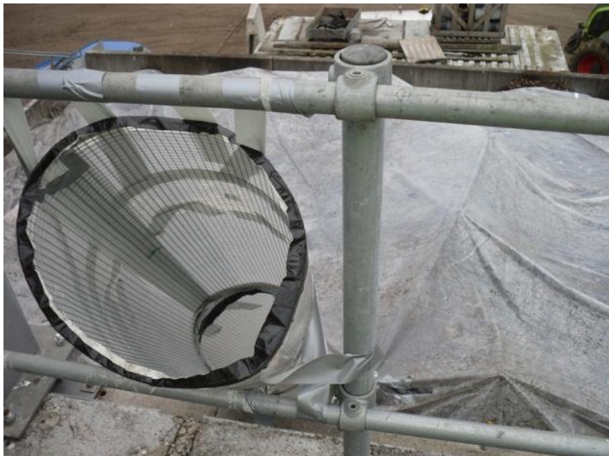
Figure 5. Main tests covering entire biofilter surface with single outlet chimney
