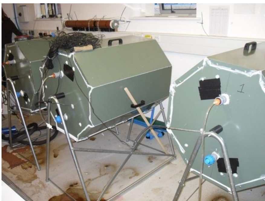
Figure 6. Composting units used for odour production.
