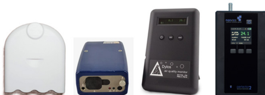
Figure 5. Handheld sensors deployed during community monitoring. From left to right: Airbeam 3 for PM 1 , PM 2.5 , PM 10 ; MicroAeth (AE-51) for black carbon; Dylos DC1700-PM for PM 2.5 and; Partector 2 for ultrafine particle number and mass.
